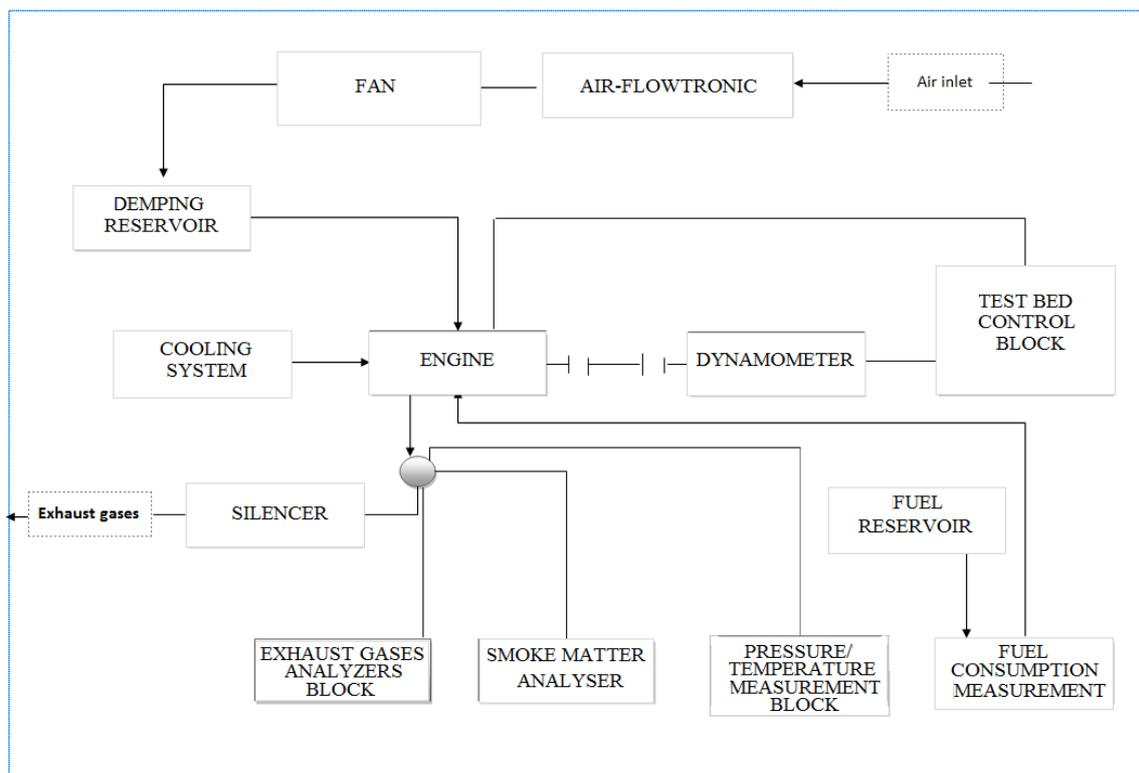
Fig. 1. The lay-out of the research test bed
