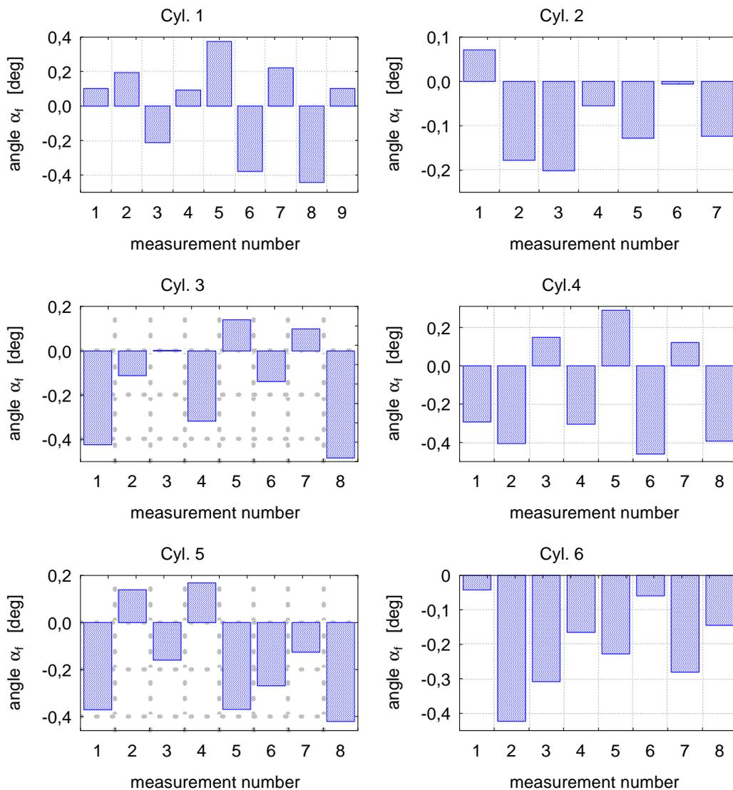
Fig. 4. The results of angle calculation. The values of the individual thermodynamic TDC and encoder's TDC differences in degrees.
