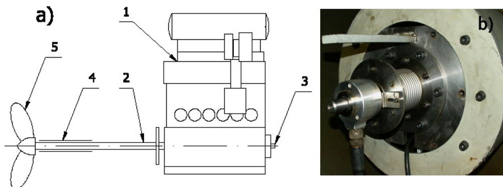
Fig. 1. The propulsion plant: a) Schematic diagram; 1-Main engine; 2-Propulsion shaft; .3-Rotary incremental encoder; 4-Stern tube with stern bearings; 5-Propeller; b) Encoder attached to the crankshaft
