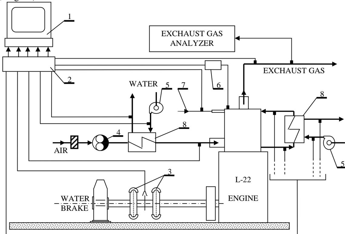
Fig.1. A schematic diagram of the laboratory stand: 1 – a recording computer, 2 – A/C converter, 3 – rubber flexible couplings, 4 – Roots' blower, 5 – a fresh water pump, 6 – an electronic indicator of pressure, 7 – fuel installation, 8 – a heat exchanger
