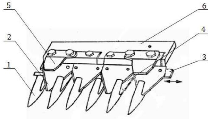
Fig. 1. An example design of a scissor-fingers cutting unit [3]:
