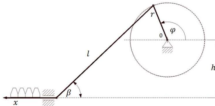
Fig 3. Schematic of an asymmetric crank mechanism:
